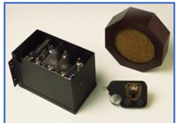
This reproduction of Motorola's first car radio, 1930's model 5T71, included (left to right) a radio receiver, tuning control and speaker.
