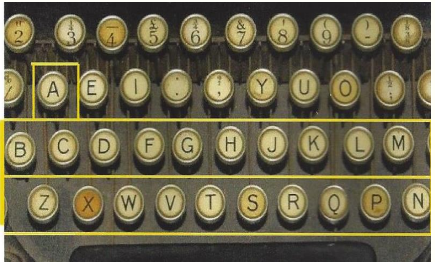
Above is the key board arrangement on the first typewriters. Notice (framed in yellow lines) that the keys were organized pretty much alphabetically by row. Print a copy and test your ability to type on this keyboard. GOOD LUCK!
